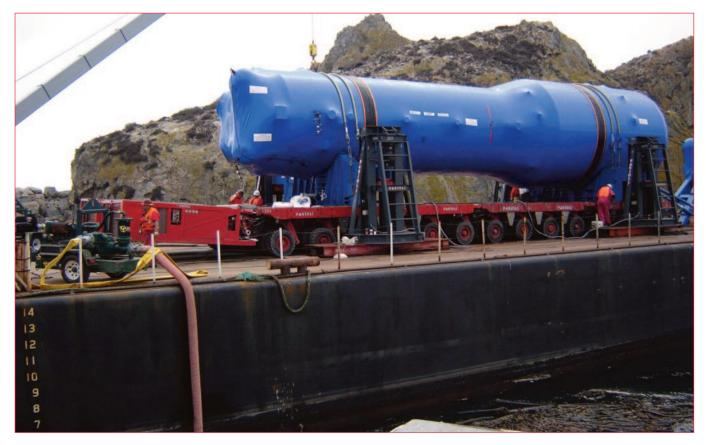
LIFTING OF A STEAM GENERATOR WEIGHING 350 TON
